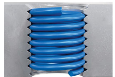
Correct installation of HELICOIL® Smart (0.25 – 0.5 x P below the surface of component)
